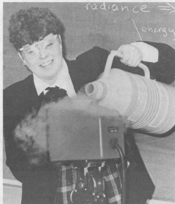
SANDIA MECHANICAL ENGINEER Beth Fuchs (8243) pours liquid nitrogen into a heat-sensing camera to illustrate how heat rather than light is detected, and how computers can be used to predict heat patterns. (Conference photos by Jim Stoots—LLNL)
